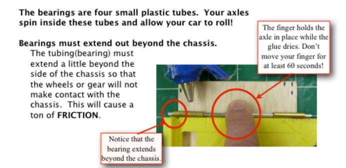
Use the T-square too to mount the bearings to the chassis. This tool creates a perfect 90 degree angel and mounts your bearings on perfectly(when used correctly) and will make your car run very straight. If your car does not run straight, it will run along the side of the track creating a lot of **FRICTION**.
