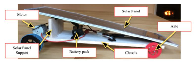
tubes that allow a metal bar (axle) to spin inside of it.
